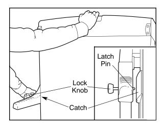
2. Hold the treadmill firmly with both hands, and lower the treadmill to the floor. Do not drop the treadmill frame to the floor. CAUTION: To decrease the possibility of injury, bend your legs and keep your back straight.
